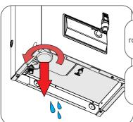
To remove filter cartridge: rotate the filter anti-clockwise.
