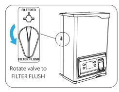
Turn ON mains water. Allow 5 litres to flow from vent outlet, to flush the filter.
