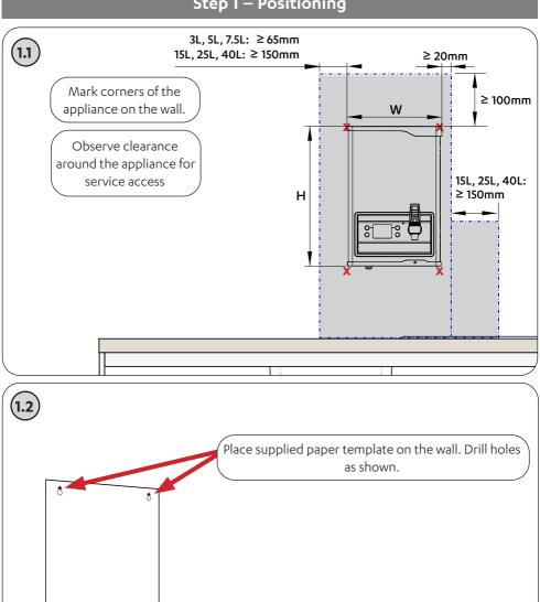
OPTION: Drill holes for concealed plumbing (water inlet, vent outlet) and electrical.
